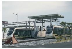
from the depot and stop by the refueling station before routine operation to urban area when refueling is required. Hydrogen is transported from Jiangmen Linkye Gas in Jiangmen City to Gaoming District of Foshan city by tanker trucks. The trams return to the depot once the operation ends at night. Service personnel then perform routine inspections and maintenance to ensure the trams are in good and safe condition for operation the next day.
